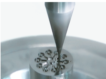
Attached to the tip of machine tools, end mills cut out materials.
