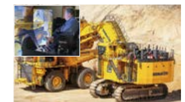
Collaborative operation by unmanned dump truck and ultra-class teleoperated hydraulic excavator (development completed in March 2023)
