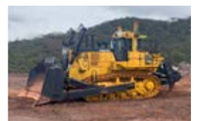
Large-scale ICT bulldozer for mining, D375Ai-8 teleoperation model
