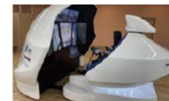
Remote control cockpit for construction equipment (mass-production verification tests underway)
