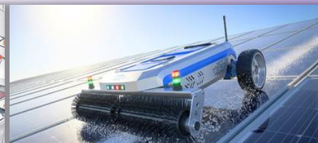
Solar panel cleaning robot → Developed a module that integrates sensing, judgment, and drive control to achieve both remote operation and autonomous navigation in outdoor environments.
